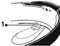
Remove the small gasket from the blue safety valve on the underside of the top cover, pull out the blue safety valve on the top and wash it in warm, soapy water.
