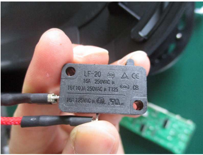
Interlock Switch: LF-20 16A T125 5E4 250V QIHONG
