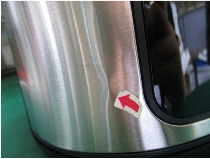
Deformation on metal plate
