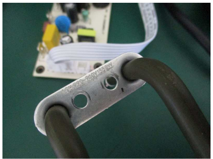
Heating element : LOH 220-240V 1550W , Dongguan Detai
